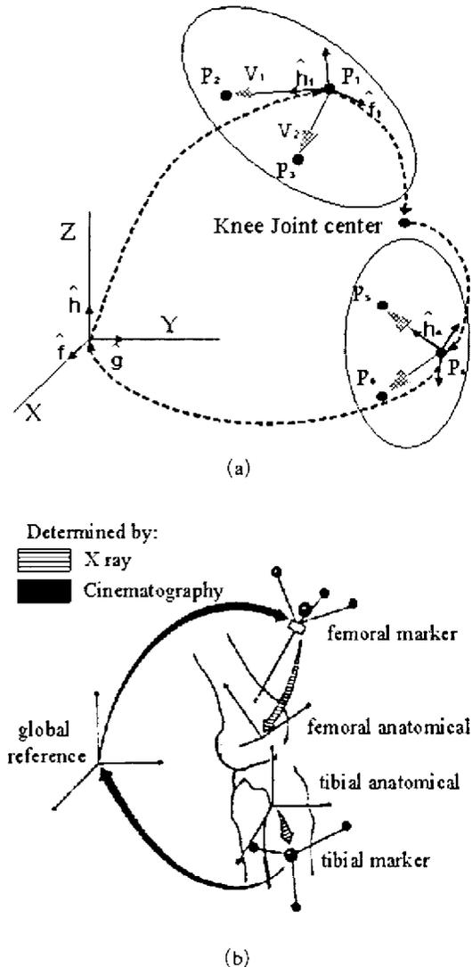
**Fig. 6** (a) Configuration of the analysis method using a relative coordinate system and (b) a configuration of the analysis method using the Bone pin marker set (Scanned picture from Lafortune et al., 1992)
